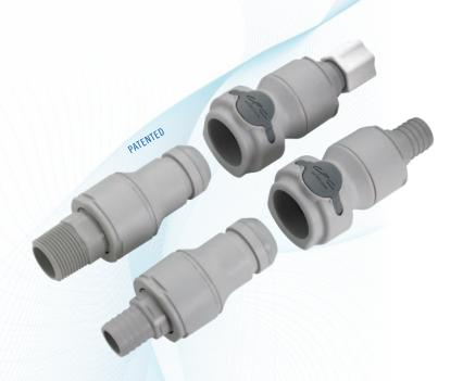
NSH Series couplings couplings are general purpose versions of our pressure-balanced, non-spill, ChemQuik® CQG06 couplings. Molded polypropylene, EPDM seals and a 100% springless and metal-free flow path provide broad chemical resistance and exceptionally high flow capacity, allowing instant disconnects (and reconnects), even under pressure. Their non-spill design virtually eliminates spills, minimizes downtime and enhances operator safety in a very low cost package.
